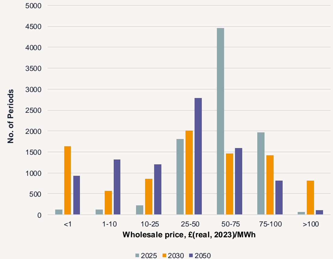
No. of periods with price at different levels for 2025, 2030 and 2050 in LCP Delta Clean Power scenario
